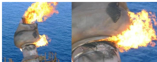
Figure 4. Visual Inspection of Flare Stack Damage Captured by UAV.
