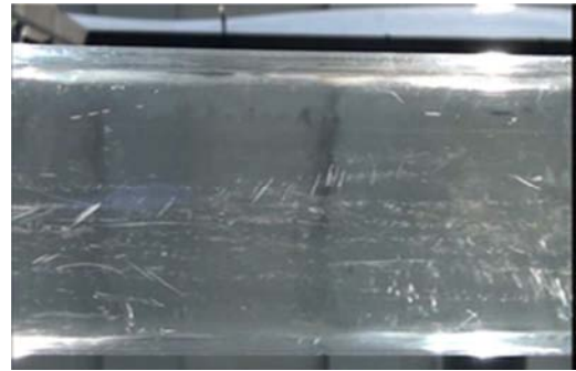
Figure 6. Suspension, V_{sl} 0.2427\text{m/s} (212microns, 200lb/1000bbl).
